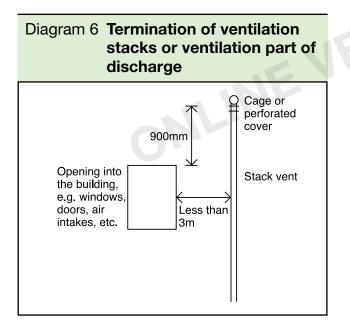
**1.32** Sizes of stack ventilation pipes – stack ventilation pipes (the dry part above the highest branch) may be reduced in size in one and two storey houses, but should be not less than 75mm.
